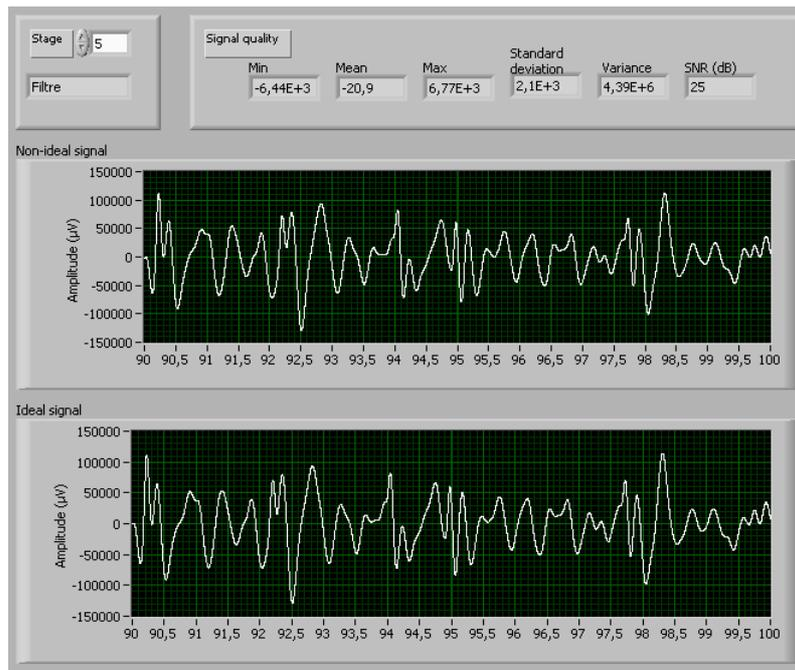
Fig 6 - The small bandpass destroys the signal shape.
