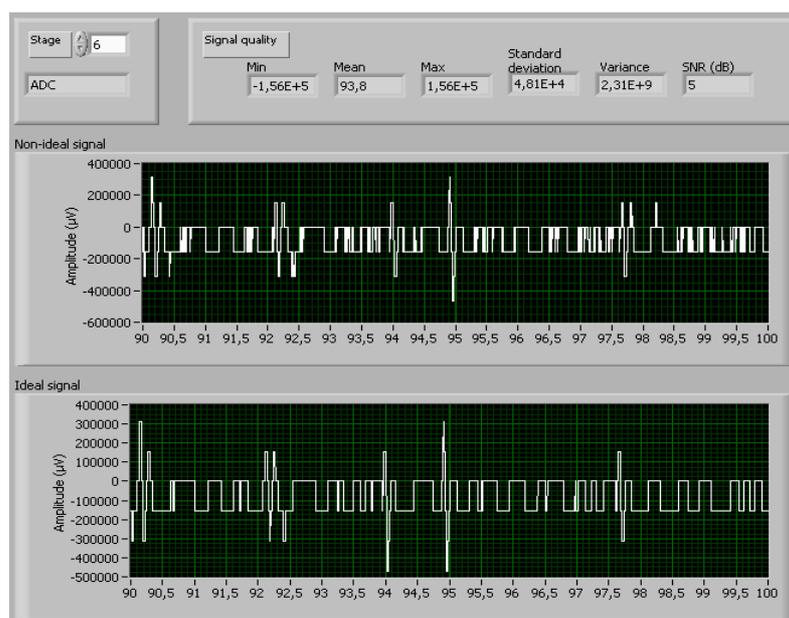
Fig 7 - The signal shape is destroyed by the 6 bit ADC.
