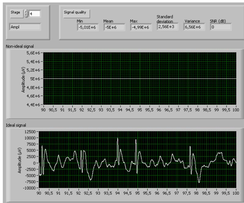
Fig 5 - A 300mV offset makes the chain saturate.
