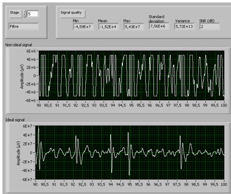
Fig 4 – The signal clips at the filter's output
